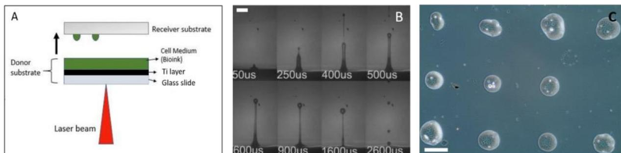
A) Sketch of LIFT process, B) Example of bioink ejection and C) Droplets with stem cells printed by LIFT
